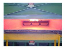
The photo shows a well-maintained 60,000# furnace. There is a tray to catch the oxides as they are raked from the furnace floor.
