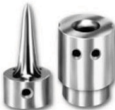
Figure 1 – A drip that gets “pinched” between the sprue bushing and the sprue post can crack the post and allow water to enter the nozzle and gooseneck!
