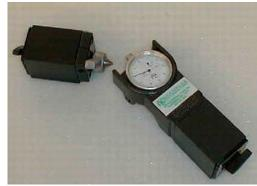
Figure 2 - Magnetic base tie bar strain gage.
