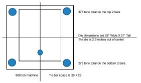
Figure 4 - Example readings for an offset die.
