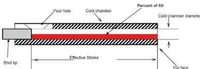
Figure 5 – Diagram of effective stroke.
