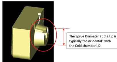
Figure 3 – Cold Chamber sprue (This is the one).
