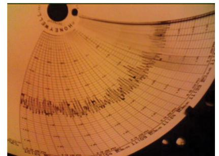
**Figure 2** - Variations of 30 PSI were recorded. This is a main line feeding 7 machines. The line from the compressor was 3 sizes smaller than the manifold.
